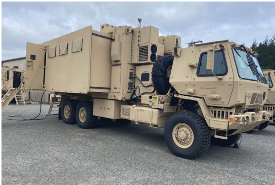
An M1087 Expandable Van Shelter houses the Command Post Integrated Infrastructure System under operational test by the 2nd Infantry Division's 2nd Stryker Brigade Combat Team at Joint Base Lewis-McChord, Washington. (Photo by Sgt. 1st Class Frederick E. Estep, U.S. Army Operational Test Command)
